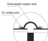
b, the use of gold belt/wire bonding interconnect width of the gold belt is less than the width of the microstrip circuit, no multiple bonding is allowed, the bonding quality should meet the requirements of GJB548B method 2017.1 Article 3.1.5, the bonding strength should meet the requirements of GJB548B method 2011.1 and 2023.2.
