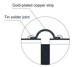
b, the use of gold belt/wire bonding interconnect, the width of the gold belt is less than the width of the microstrip circuit, no multiple bonding is allowed, the bonding quality should meet the requirements of GJB548B method 2017.1 Article 3.1.5, the bonding strength should meet the requirements of GJB548B method 2011.1 and 2023.2.
