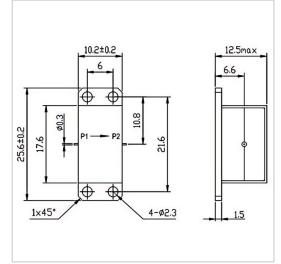
RF Solution offer a wide selection of Drop in Isolator for global customers. WG1017C is a Drop in Isolator in Frequency Range of 17.0~31.0 GHz. It is made of high quality materials under a high standard, the Bandwidth Max of this product is 38%, Insertion Loss Max is 0.80~1.00 dB and Isolation Min is 20.0 dB. The component has a good working performance and stability, it is ideal for handling a Forward Power of 10 W.
