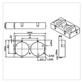
RF Solution offer a wide selection of Dual Junction Circulator for global customers. WHH9050X is a Dual Junction Circulator in Frequency Range of 300~1250 MHz. It is made of high quality materials under a high standard, the Bandwidth Max of this product is 20%, Insertion Loss Max is 0.60~1.60 dB and Isolation Min is 32.0~50.0 dB. The component has a good working performance and stability, it is ideal for handling a Forward Power of 300 W.
