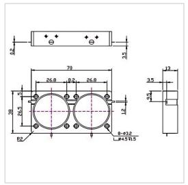
RF Solution offer a wide selection of Dual Junction Circulator for global customers. WHH7038X is a Dual Junction Circulator in Frequency Range of 400~1850 MHz. It is made of high quality materials under a high standard, the Bandwidth Max of this product is 20%, Insertion Loss Max is 0.50~1.40 dB and Isolation Min is 32.0~50.0 dB. The component has a good working performance and stability, it is ideal for handling a Forward Power of 300 W.
