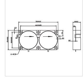
RF Solution offer a wide selection of Dual Junction Circulator for global customers. WHH5025X is a Dual Junction Circulator in Frequency Range of 250~2700 MHz. It is made of high quality materials under a high standard, the Bandwidth Max of this product is 15%, Insertion Loss Max is 0.40~1.00 dB and Isolation Min is 36.0~50.0 dB. The component has a good working performance and stability, it is ideal for handling a Forward Power of 250 W.
