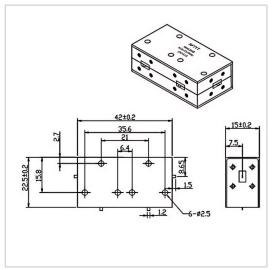
RF Solution offer a wide selection of Dual Junction Circulator for global customers. WHH4223B is a Dual Junction Circulator in Frequency Range of 4.0~8.0 GHz. It is made of high quality materials under a high standard, the Bandwidth Max of this product is 100%, Insertion Loss Max is 0.80~1.20 dB and Isolation Min is 36.0~38.0 dB. The component has a good working performance and stability, it is ideal for handling a Forward Power of 30 W.
