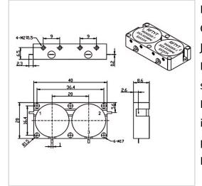
RF Solution offer a wide selection of Dual Junction Circulator for global customers. WHH4020X is a Dual Junction Circulator in Frequency Range of 600~2700 MHz. It is made of high quality materials under a high standard, the Bandwidth Max of this product is 15%, Insertion Loss Max is 0.60~1.00 dB and Isolation Min is 36.0~46.0 dB. The component has a good working performance and stability, it is ideal for handling a Forward Power of 100 W.
