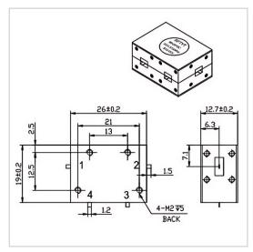
RF Solution offer a wide selection of Dual Junction Circulator for global customers. WHH2619C is a Dual Junction Circulator in Frequency Range of 6.0~12.0 GHz. It is made of high quality materials under a high standard, the Bandwidth Max of this product is 100%, Insertion Loss Max is 1.20 dB and Isolation Min is 34.0~36.0 dB. The component has a good working performance and stability, it is ideal for handling a Forward Power of 30 W.
