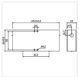
RF Solution offer a wide selection of Dual Junction Circulator for global customers. WHH14566K is a Dual Junction Circulator in Frequency Range of 1.0~2.0 GHz. It is made of high quality materials under a high standard, the Bandwidth Max of this product is 100%, Insertion Loss Max is 0.65~1.30 dB and Isolation Min is 17.0~32.0 dB. The component has a good working performance and stability, it is ideal for handling a Forward Power of 100 W.
