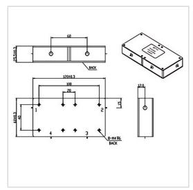
RF Solution offer a wide selection of Dual Junction Circulator for global customers. WHH12060E is a Dual Junction Circulator in Frequency Range of 80~230 MHz. It is made of high quality materials under a high standard, the Bandwidth Max of this product is 30%, Insertion Loss Max is 0.80~2.00 dB and Isolation Min is 36.0~46.0 dB. The component has a good working performance and stability, it is ideal for handling a Forward Power of 150 W.
