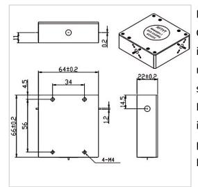
RF Solution offer a wide selection of Drop in Circulator for global customers. WH6466H is a Drop in Circulator in Frequency Range of 30~40 MHz. It is made of high quality materials under a high standard, the Bandwidth Max of this product is 5%, Insertion Loss Max is 1.50~2.00 dB and Isolation Min is 18.0~20.0 dB. The component has a good working performance and stability, it is ideal for handling a Power of 50 W.
