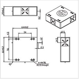
RF Solution offer a wide selection of Drop in Circulator for global customers. WH6466E is a Drop in Circulator in Frequency Range of 136~240 MHz. It is made of high quality materials under a high standard, the Bandwidth Max of this product is 20%, Insertion Loss Max is 0.45~0.80 dB and Isolation Min is 18.0~23.0 dB. The component has a good working performance and stability, it is ideal for handling a Power of 150 W.
