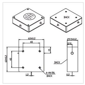
RF Solution offer a wide selection of Drop in Circulator for global customers. WH6060E is a Drop in Circulator in Frequency Range of 40~400 MHz. It is made of high quality materials under a high standard, the Bandwidth Max of this product is 50%, Insertion Loss Max is 0.40~1.60 dB and Isolation Min is 18.0~23.0 dB. The component has a good working performance and stability, it is ideal for handling a Forward Power of 50 W.
