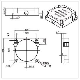
RF Solution offer a wide selection of Drop in Circulator for global customers. WH5050X is a Drop in Circulator in Frequency Range of 160~330 MHz. It is made of high quality materials under a high standard, the Bandwidth Max of this product is 20%, Insertion Loss Max is 0.30~0.90 dB and Isolation Min is 18.0~23.0 dB. The component has a good working performance and stability, it is ideal for handling a Power of 300 W.
