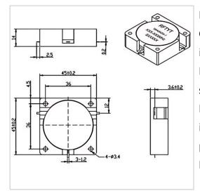
RF Solution offer a wide selection of Drop in Circulator for global customers. WH4545X is a Drop in Circulator in Frequency Range of 250~1400 MHz. It is made of high quality materials under a high standard, the Bandwidth Max of this product is 35%, Insertion Loss Max is 0.30~0.80 dB and Isolation Min is 16.0~25.0 dB. The component has a good working performance and stability, it is ideal for handling a Power of 200 W.
