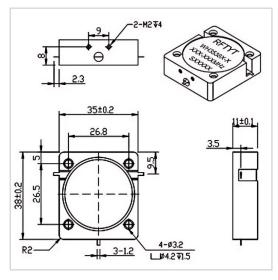
RF Solution offer a wide selection of Drop in Circulator for global customers. WH3538X is a Drop in Circulator in Frequency Range of 300~1850 MHz. It is made of high quality materials under a high standard, the Bandwidth Max of this product is 30%, Insertion Loss Max is 0.20~0.80 dB and Isolation Min is 17.0~25.0 dB. The component has a good working performance and stability, it is ideal for handling a Power of 300 W.
