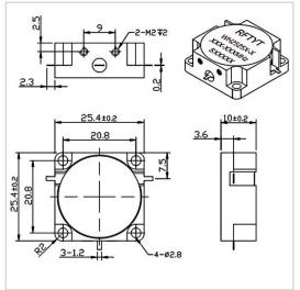
RF Solution offer a wide selection of Drop in Circulator for global customers. WH2525X is a Drop in Circulator in Frequency Range of 350~4300 MHz. It is made of high quality materials under a high standard, the Bandwidth Max of this product is 15%, Insertion Loss Max is 0.20~0.70 dB and Isolation Min is 16.0~25.0 dB. The component has a good working performance and stability, it is ideal for handling a Power of 50 W.
