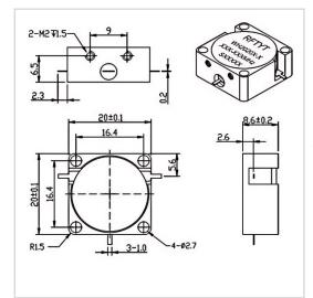
RF Solution offer a wide selection of Drop in Circulator for global customers. WH2020X is a Drop in Circulator in Frequency Range of 700~4000 MHz. It is made of high quality materials under a high standard, the Bandwidth Max of this product is 15%, Insertion Loss Max is 0.30~0.60 dB and Isolation Min is 18.0~23.0 dB. The component has a good working performance and stability, it is ideal for handling a Power of 100 W.
