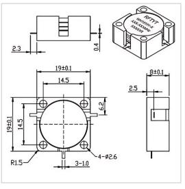
RF Solution offer a wide selection of Drop in Circulator for global customers. WH1919Y is a Drop in Circulator in Frequency Range of 850~5000 MHz. It is made of high quality materials under a high standard, the Bandwidth Max of this product is 10%, Insertion Loss Max is 0.30~0.50 dB and Isolation Min is 18.0~23.0 dB. The component has a good working performance and stability, it is ideal for handling a Power of 50 W.
