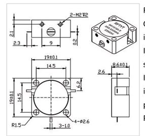
RF Solution offer a wide selection of Drop in Circulator for global customers. WH1919X is a Drop in Circulator in Frequency Range of 850~5000 MHz. It is made of high quality materials under a high standard, the Bandwidth Max of this product is 10%, Insertion Loss Max is 0.30~0.50 dB and Isolation Min is 18.0~23.0 dB. The component has a good working performance and stability, it is ideal for handling a Power of 50 W.
