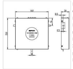
RF Solution offer a wide selection of Drop in Circulator for global customers. WH160150E is a Drop in Circulator in Frequency Range of 70~130 MHz. It is made of high quality materials under a high standard, the Bandwidth Max of this product is 2%, Insertion Loss Max is 0.30 dB and Isolation Min is 20.0~23.0 dB. The component has a good working performance and stability, it is ideal for handling a Forward Power of 1000 W.
