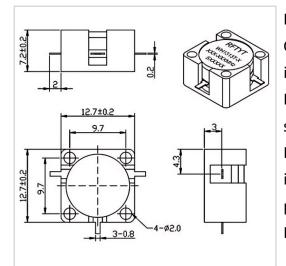
RF Solution offer a wide selection of Drop in Circulator for global customers. WH1313T is a Drop in Circulator in Frequency Range of 800~7000 MHz. It is made of high quality materials under a high standard, the Bandwidth Max of this product is 10%, Insertion Loss Max is 0.30~0.50 dB and Isolation Min is 18.0~23.0 dB. The component has a good working performance and stability, it is ideal for handling a Power of 50 W.
