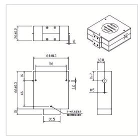
RF Solution offer a wide selection of Drop in Isolator for global customers. WG6466K is a Drop in Isolator in Frequency Range of 1.0~2.0 GHz. It is made of high quality materials under a high standard, the Bandwidth Max of this product is 100%, Insertion Loss Max is 0.70 dB and Isolation Min is 17.0 dB. The component has a good working performance and stability, it is ideal for handling a Forward Power of 100 W.
