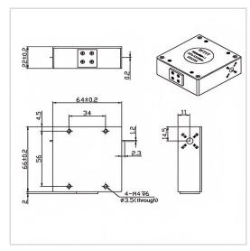
RF Solution offer a wide selection of Drop in Isolator for global customers. WG6466H is a Drop in Isolator in Frequency Range of 30.0~40.0 MHz. It is made of high quality materials under a high standard, the Bandwidth Max of this product is 5%, Insertion Loss Max is 1.50~2.00 dB and Isolation Min is 18.0~20.0 dB. The component has a good working performance and stability, it is ideal for handling a Forward Power of 50 W.
