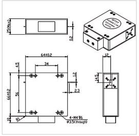
RF Solution offer a wide selection of Drop in Isolator for global customers. WG6466E is a Drop in Isolator in Frequency Range of 100~200 MHz. It is made of high quality materials under a high standard, the Bandwidth Max of this product is 20%, Insertion Loss Max is 0.50~0.80 dB and Isolation Min is 18.0~20.0 dB. The component has a good working performance and stability, it is ideal for handling a Forward Power of 300 W.
