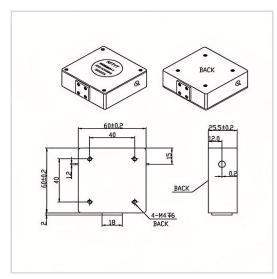
RF Solution offer a wide selection of Drop in Isolator for global customers. WG6060E is a Drop in Isolator in Frequency Range of 45~400 MHz. It is made of high quality materials under a high standard, the Bandwidth Max of this product is 50%, Insertion Loss Max is 0.40~1.60 dB and Isolation Min is 18.0~23.0 dB. The component has a good working performance and stability, it is ideal for handling a Forward Power of 100 W.
