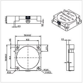
RF Solution offer a wide selection of Drop in Isolator for global customers. WG5050X is a Drop in Isolator in Frequency Range of 160~330 MHz. It is made of high quality materials under a high standard, the Bandwidth Max of this product is 20%, Insertion Loss Max is 0.50~0.80 dB and Isolation Min is 18.0~20.0 dB. The component has a good working performance and stability, it is ideal for handling a Forward Power of 300 W.
