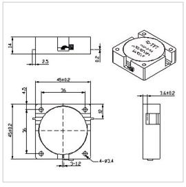
RF Solution offer a wide selection of Drop in Isolator for global customers. WG4545X is a Drop in Isolator in Frequency Range of 250~1400 MHz. It is made of high quality materials under a high standard, the Bandwidth Max of this product is 35%, Insertion Loss Max is 0.30~0.80 dB and Isolation Min is 15.0~23.0 dB. The component has a good working performance and stability, it is ideal for handling a Forward Power of 100 W.
