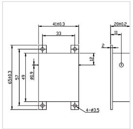
RF Solution offer a wide selection of Drop in Isolator for global customers. WG4149A is a Drop in Isolator in Frequency Range of  $300\sim1000$  MHz. It is made of high quality materials under a high standard, the Bandwidth Max of this product is 20%, Insertion Loss Max is  $0.60\sim1.20$  dB and Isolation Min is  $14.0\sim20.0$  dB. The component has a good working performance and stability, it is ideal for handling a Forward Power of 100 W.
