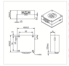
RF Solution offer a wide selection of Drop in Isolator for global customers. WG4040A is a Drop in Isolator in Frequency Range of 1.50~3.5 GHz. It is made of high quality materials under a high standard, the Bandwidth Max of this product is 100%, Insertion Loss Max is 0.60~0.70 dB and Isolation Min is 17.0~18.0 dB. The component has a good working performance and stability, it is ideal for handling a Forward Power of 150 W.
