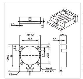
RF Solution offer a wide selection of Drop in Isolator for global customers. WG3546X-30dB is a Drop in Isolator in Frequency Range of 300~1850 MHz. It is made of high quality materials under a high standard, the Bandwidth Max of this product is 30%, Insertion Loss Max is 0.20~0.80 dB and Isolation Min is 16.0~25.0 dB. The component has a good working performance and stability, it is ideal for handling a Forward Power of 100 W.
