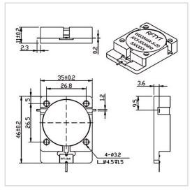
RF Solution offer a wide selection of Drop in Isolator for global customers. WG3546X-20dB is a Drop in Isolator in Frequency Range of  $300\sim1850$  MHz. It is made of high quality materials under a high standard, the Bandwidth Max of this product is 30%, Insertion Loss Max is  $0.30\sim0.80$  dB and Isolation Min is  $16.0\sim25.0$  dB. The component has a good working performance and stability, it is ideal for handling a Forward Power of 100 W.
