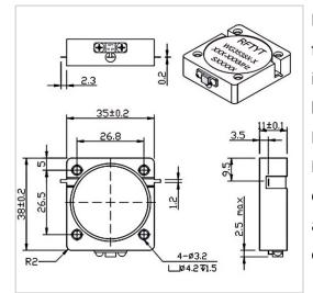
RF Solution offer a wide selection of Drop in Isolator for global customers. WG3538X is a Drop in Isolator in Frequency Range of 300~1850 MHz. It is made of high quality materials under a high standard, the Bandwidth Max of this product is 30%, Insertion Loss Max is 0.25~0.80 dB and Isolation Min is 16.0~25.0 dB. The component has a good working performance and stability, it is ideal for handling a Forward Power of 200 W.
