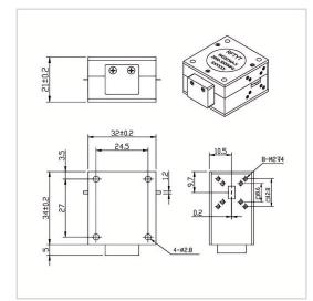
RF Solution offer a wide selection of Drop in Isolator for global customers. WG3234B is a Drop in Isolator in Frequency Range of 2.0~4.0 GHz. It is made of high quality materials under a high standard, the Bandwidth Max of this product is 100%, Insertion Loss Max is 0.40~0..50 dB and Isolation Min is 18.0~20.0 dB. The component has a good working performance and stability, it is ideal for handling a Forward Power of 150 W.
