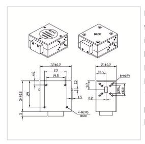
RF Solution offer a wide selection of Drop in Isolator for global customers. WG3234A is a Drop in Isolator in Frequency Range of 2.0~4.0 GHz. It is made of high quality materials under a high standard, the Bandwidth Max of this product is 100%, Insertion Loss Max is 0.50~0.60 dB and Isolation Min is 18.0~19.0 dB. The component has a good working performance and stability, it is ideal for handling a Forward Power of 150 W.
