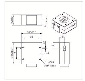
RF Solution offer a wide selection of Drop in Isolator for global customers. WG3030B is a Drop in Isolator in Frequency Range of 2.0~6.0 GHz. It is made of high quality materials under a high standard, the Bandwidth Max of this product is 100%, Insertion Loss Max is 0.85~1.70 dB and Isolation Min is 12.0 dB. The component has a good working performance and stability, it is ideal for handling a Forward Power of 50 W.
