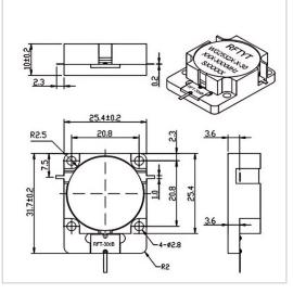
RF Solution offer a wide selection of Drop in Isolator for global customers. WG2532X-30dB is a Drop in Isolator in Frequency Range of 350~4300 MHz. It is made of high quality materials under a high standard, the Bandwidth Max of this product is 25%, Insertion Loss Max is 0.20~0.70 dB and Isolation Min is 17.0~25.0 dB. The component has a good working performance and stability, it is ideal for handling a Forward Power of 100/200 W.
