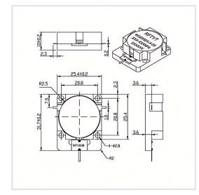
RF Solution offer a wide selection of Drop in Isolator for global customers. WG2532X-20dB is a Drop in Isolator in Frequency Range of 350~4300 MHz. It is made of high quality materials under a high standard, the Bandwidth Max of this product is 25%, Insertion Loss Max is 0.25~0.70 dB and Isolation Min is 17.0~25.0 dB. The component has a good working performance and stability, it is ideal for handling a Forward Power of 100/200 W.
