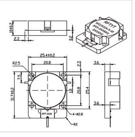
RF Solution offer a wide selection of Drop in Isolator for global customers. WG2532X-100W is a Drop in Isolator in Frequency Range of 350~4300 MHz. It is made of high quality materials under a high standard, the Bandwidth Max of this product is 25%, Insertion Loss Max is 0.20~0.70 dB and Isolation Min is 17.0~25.0 dB. The component has a good working performance and stability, it is ideal for handling a Forward Power of 100/200 W.
