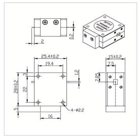
RF Solution offer a wide selection of Drop in Isolator for global customers. WG2528C is a Drop in Isolator in Frequency Range of  $3.0\sim6.0$  GHz. It is made of high quality materials under a high standard, the Bandwidth Max of this product is 100%, Insertion Loss Max is  $0.40\sim0.50$  dB and Isolation Min is  $18.0\sim20.0$  dB. The component has a good working performance and stability, it is ideal for handling a Forward Power of 150 W.
