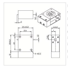
RF Solution offer a wide selection of Drop in Isolator for global customers. WG2528C-100W is a Drop in Isolator in Frequency Range of 3.0~6.0 GHz. It is made of high quality materials under a high standard, the Bandwidth Max of this product is 100%, Insertion Loss Max is 0.40~0.50 dB and Isolation Min is 18.0~20.0 dB. The component has a good working performance and stability, it is ideal for handling a Forward Power of 100 W.
