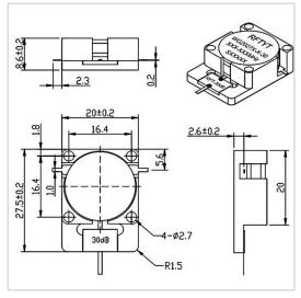
RF Solution offer a wide selection of Drop in Isolator for global customers. WG2027X-30dB is a Drop in Isolator in Frequency Range of 700~4000 MHz. It is made of high quality materials under a high standard, the Bandwidth Max of this product is 25%, Insertion Loss Max is 0.30~0.50 dB and Isolation Min is 18.0~23.0 dB. The component has a good working performance and stability, it is ideal for handling a Forward Power of 100 W.
