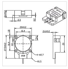
RF Solution offer a wide selection of Drop in Isolator for global customers. WG2027X-20dB is a Drop in Isolator in Frequency Range of 700~4000 MHz. It is made of high quality materials under a high standard, the Bandwidth Max of this product is 25%, Insertion Loss Max is 0.30~0.50 dB and Isolation Min is 18.0~23.0 dB. The component has a good working performance and stability, it is ideal for handling a Forward Power of 100 W.
