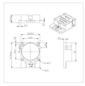
RF Solution offer a wide selection of Drop in Isolator for global customers. WG2027X-100W is a Drop in Isolator in Frequency Range of 700~4000 MHz. It is made of high quality materials under a high standard, the Bandwidth Max of this product is 25%, Insertion Loss Max is 0.30~0.50 dB and Isolation Min is 18.0~23.0 dB. The component has a good working performance and stability, it is ideal for handling a Forward Power of 100 W.
