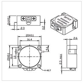
RF Solution offer a wide selection of Drop in Isolator for global customers. WG2020X is a Drop in Isolator in Frequency Range of 700~4000 MHz. It is made of high quality materials under a high standard, the Bandwidth Max of this product is 25%, Insertion Loss Max is 0.30~0.50 dB and Isolation Min is 17.0~23.0 dB. The component has a good working performance and stability, it is ideal for handling a Forward Power of 100 W.
