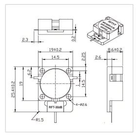
RF Solution offer a wide selection of Drop in Isolator for global customers. WG1925X-30dB is a Drop in Isolator in Frequency Range of 850~5000 MHz. It is made of high quality materials under a high standard, the Bandwidth Max of this product is 25%, Insertion Loss Max is 0.30~0.50 dB and Isolation Min is 18.0~23.0 dB. The component has a good working performance and stability, it is ideal for handling a Forward Power of 100 W.
