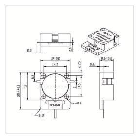
RF Solution offer a wide selection of Drop in Isolator for global customers. WG1925X-20dB is a Drop in Isolator in Frequency Range of 850~5000 MHz. It is made of high quality materials under a high standard, the Bandwidth Max of this product is 25%, Insertion Loss Max is 0.30~0.50 dB and Isolation Min is 18.0~23.0 dB. The component has a good working performance and stability, it is ideal for handling a Forward Power of 100 W.
