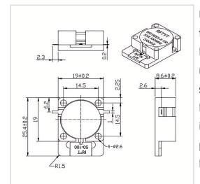
RF Solution offer a wide selection of Drop in Isolator for global customers. WG1925X-100W is a Drop in Isolator in Frequency Range of 850~5000 MHz. It is made of high quality materials under a high standard, the Bandwidth Max of this product is 25%, Insertion Loss Max is 0.30~0.60 dB and Isolation Min is 18.0~23.0 dB. The component has a good working performance and stability, it is ideal for handling a Forward Power of 100 W.
