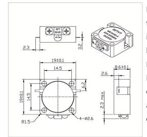
RF Solution offer a wide selection of Drop in Isolator for global customers. WG1919X is a Drop in Isolator in Frequency Range of 850~5000 MHz. It is made of high quality materials under a high standard, the Bandwidth Max of this product is 25%, Insertion Loss Max is 0.30~0.50 dB and Isolation Min is 18.0~23.0 dB. The component has a good working performance and stability, it is ideal for handling a Forward Power of 100 W.
